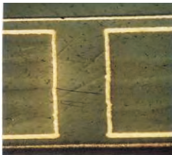
Core board thickness: 0.65mm buried via hole diameter: \varnothing 0.30mm Aspect ratio: 2.2
